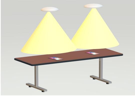
Fig. 5. Representation of the testbed used for the experiments, with one large classroom table and two VLC-enabled LED lighting sources.
