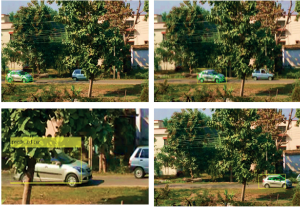
Fig. 11. Tracking of the vehicle before, during and after undergoing partial occlusion in presence of other vehicle.
