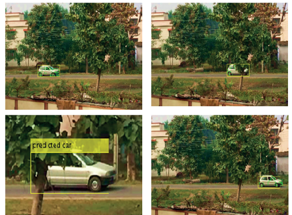
Fig. 10. Tracking of the vehicle before, during and after undergoing partial occlusion.
