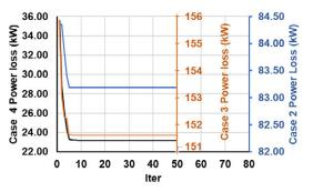
Fig. 13. Convergence characteristics of the WOA for 69-bus at different case studies.
