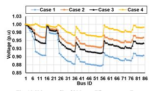
Fig. 15. Voltage profile of 85-bus at different case studies.
