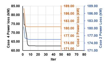
Fig. 16. Convergence characteristics of the WOA for 85-bus at different case studies.
