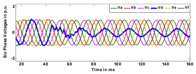
Fig. 2. Six-phase voltages during 'D-g' phase to ground fault.
