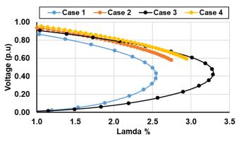
Fig. 17. PV curve for 85-bus at different case studies.
