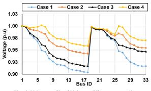
Fig. 9. Voltage profile of 33-bus at different case studies.
