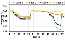
Fig. 12. Voltage profile of 69-bus at different case studies.
