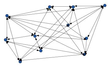
Fig. 1. The point-to-point architecture of air routes.
