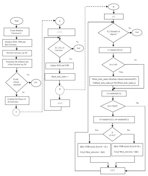
Fig. 1. General Flowchart representation of Multi-verse Optimization algorithm.
