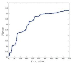
Fig. 9. The convergence plot of the proposed model
