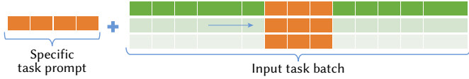
Fig. 1. Example of how a specific task prompt is added along the input tasks.
